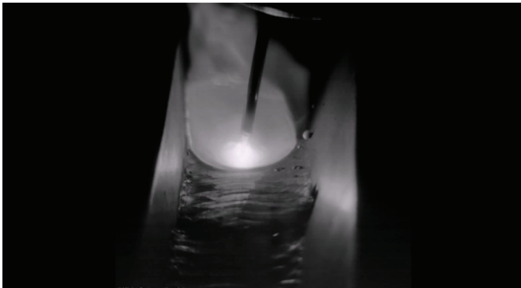
Fillet Welding of Groove in Nuclear Vessel
