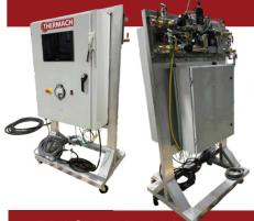
The AT-3200 Console is built for versatility, allowing the system to interface with and control multiple gas trains in order to manage complex systems. The carrier gas flows are managed by the controller, allowing for multiple powder feeders to be controlled simultaneously.
