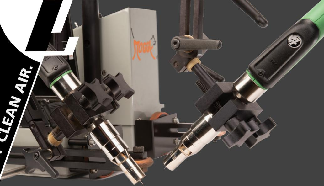
The Translas fume extraction system reduces the amount of welding fumes and particulates in the workplace to less than 1 mg/m3 during an 8-hour working day.
